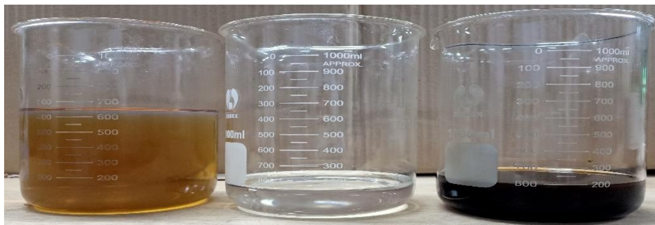
Figure 2. Physical appearance of test fuels (a)DF (b) N-pentanol (c) Used cooking oil
